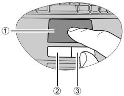
The touchpad with its buttons is a pointing device that functions as an optional external mouse, which can perform navigation, scrolling and selection functions. The components of the touchpad are described as follows.
