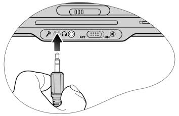
Connect a microphone to the microphone socket to record sounds.
