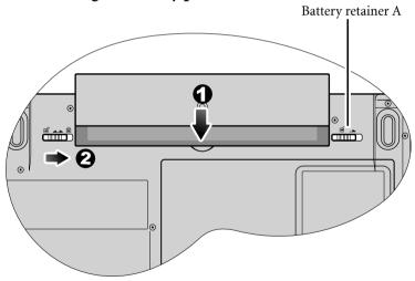
Turn your Joybook upside down and put it on a soft clean cloth. With the label side of the battery pack facing down, slide it gently into the battery compartment until it snaps into place (1). Move the battery retainer A to the left as shown to lock the battery pack into place (2).
