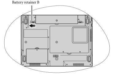
3. Slide the battery retainer A to the unlock position (1) and, while still holding the retainer, pull the battery away from its compartment (2).
