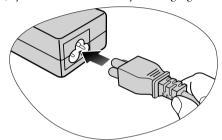
Connect the power cord to the power adapter.
