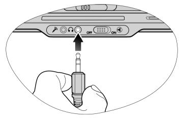
Connect an earphone to the audio output socket to output sounds.
