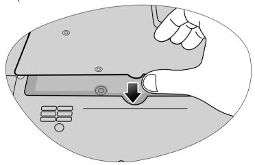
9. Use a screwdriver to secure it with the screws.
