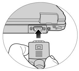
Connect an external display device (such as a monitor or projector) to the 15-pin D-sub video socket of your Joybook.
