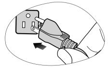
Connect the power cord to a wall outlet. The Joybook will automatically start charging the battery.
