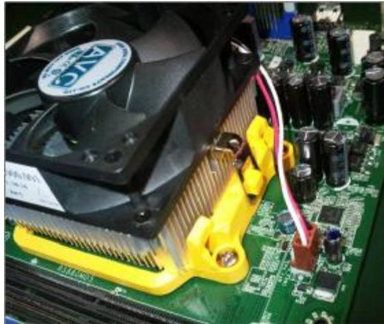
4.4 Fix two side buckles and rotate latch of CPU Cooler to MB.
