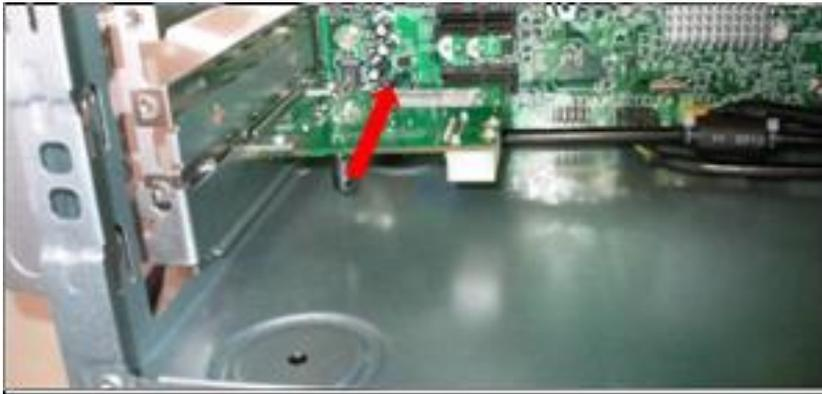
**8.5** Combination the 15 PIN POWER cable with SATA Connect
