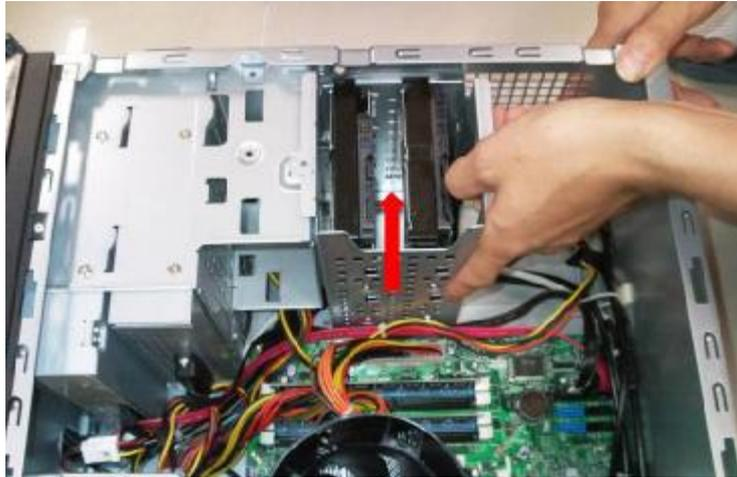
4.4 Disconnect the eight screws fixed in HDD cage side.
