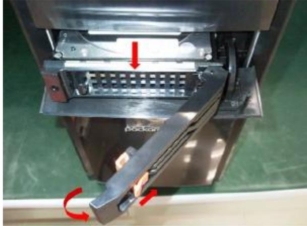
9.3 Rotate rubber pin in Carrier and removing HDD
