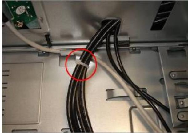
10.2 Press ten hooks on TOP Bezel , disconnect cable and remove it
