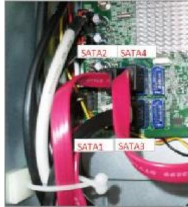
**6.11** HDD/ODD install rule
