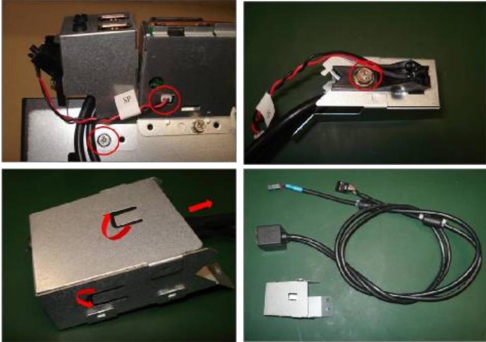
**10.6** Disconnect the two screws fastening Card Reader bracket to the case, disconnect the button cable and the screw
