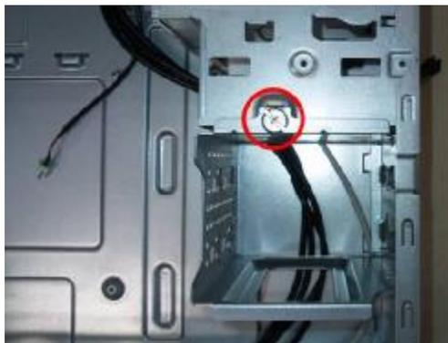
2.4 Pulling out the HDD cage
