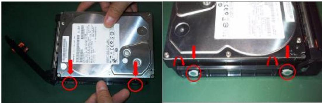
**6.6 Insert the HDD Carrier to Chassis**
