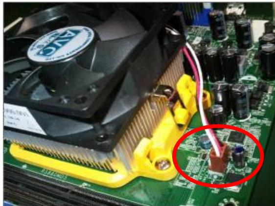
7.8 Release two side buckles and rotate latch of CPU Cooler then remove it
