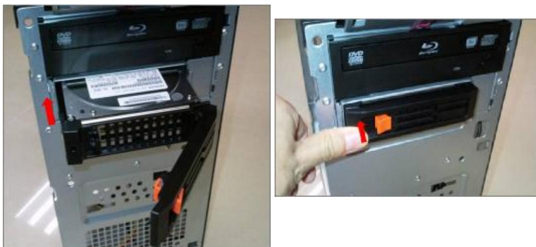
6.7 Pulling in HDD Carrier SATA cable on Motherboard
