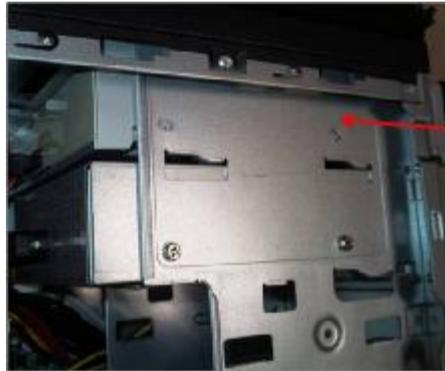
6.3 Fix two screws for each ODD and pulling in ODD SATA cable on Motherboard
