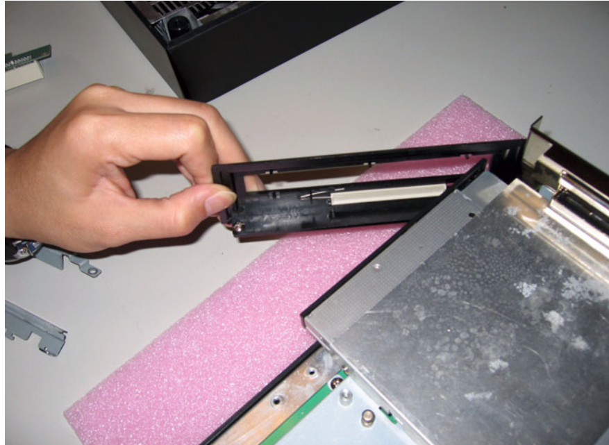
Figure A.16 Removing the CD-ROM / PCMCIA slot cover.
