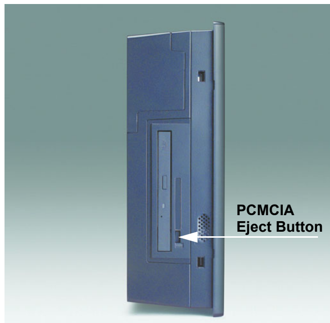
Figure 3.2 Inserting and ejecting a PCMCIA card
