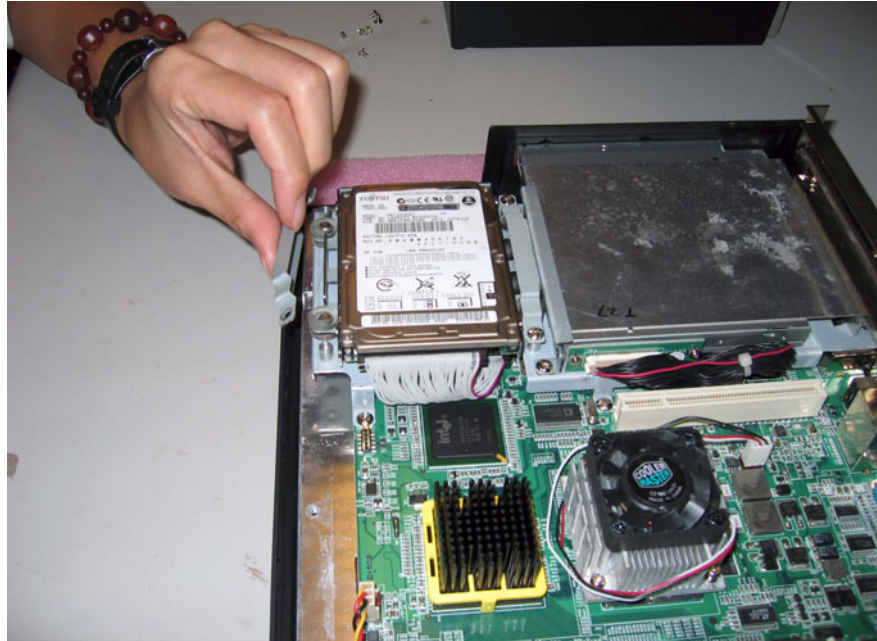
Figure A.8 Unfastening the HDD module
