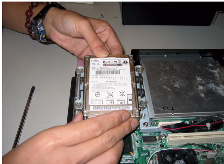
Figure A.9 Removing the HDD
