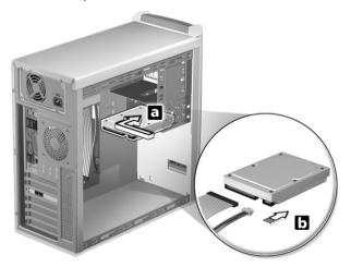
5 Secure it with the four screws you removed earlier.
