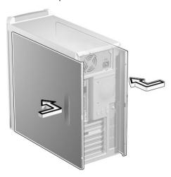
2 Secure the side panels with the four screws you removed earlier.
