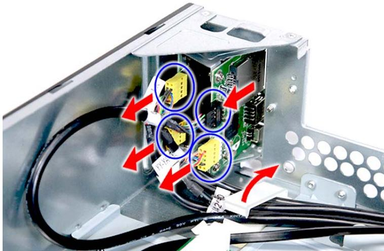
9. Open the cable retention clip and disconnect the other end of the USB, 1394, and audio cables from the mainboard.
