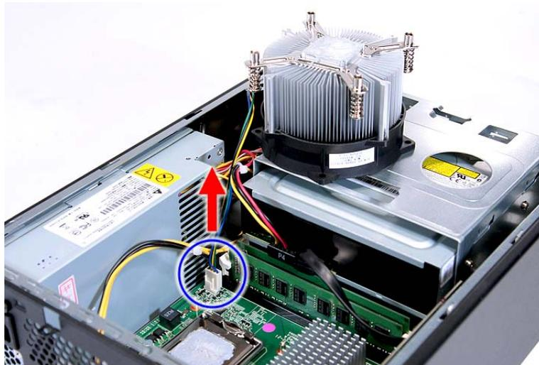
5. Remove the heat sink fan assembly from the chassis then lay it down in an upright position—with the thermal patch facing upward. Do not let the thermal patch on the heat sink fan assembly touch the work surface.
