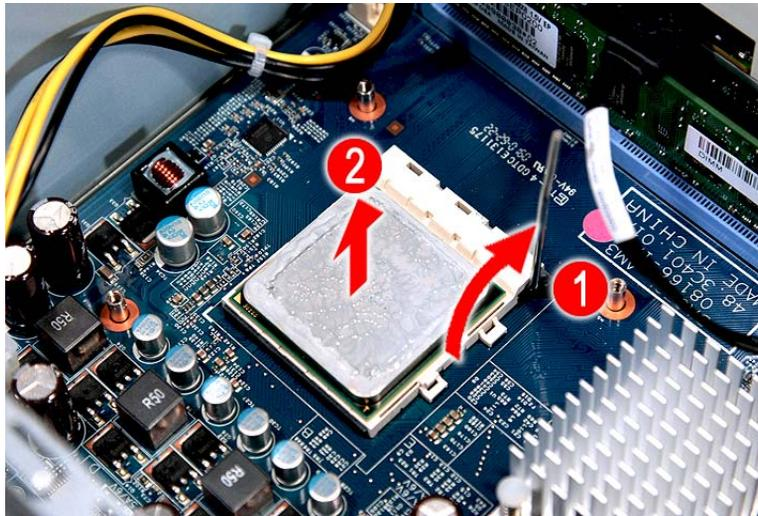
**IMPORTANT:** If you are going to install a new processor, note the arrow on the corner to make sure the processor is properly oriented over the socket.
