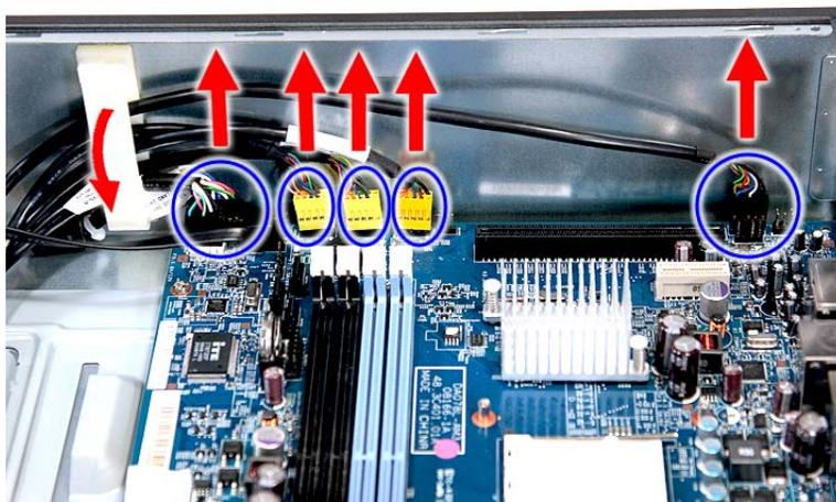
10. Remove the front I/O and card reader board bracket.
