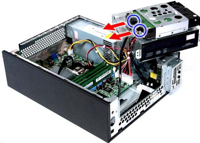
**(5).** Remove the HDD-ODD bracket.
