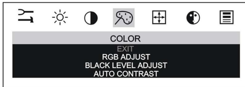
When you choose the Color option from the OSD, this will bring up a sub-menu that allows you to adjust the RGB or Black Level color balance for your display. Use the ◀/left and ▶/right arrow buttons to scroll through the color menu.
