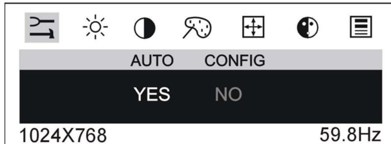
To perform an Auto Config, press the ◀/left arrow key once then press SELECT. The Main Menu item Auto Config is used to adjust the configuration of the phase clock vertical and horizontal position automatically. A confirmation box is displayed to confirm the user selection. The default selection in the box is NO and is highlighted by a red bar.
