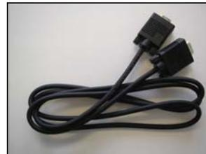
**9-pin RS-232 serial communication cable (if applicable)**
