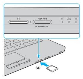
3 Carefully slide the memory card into the slot until it clicks into place. Do not force the card into the slot.
