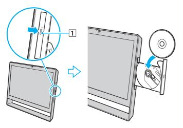
Do not exert pressure on the drive tray. Be sure to hold the back of the drive tray when placing/removing a disc onto/from the drive tray.
