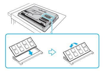
Do not touch any components on the motherboard other than the memory module.
