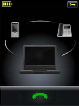
Figure 33: A disconnected target phone is shown greyed out on the touchscreen.
