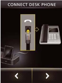
Figure 21: Connect to the handset port
