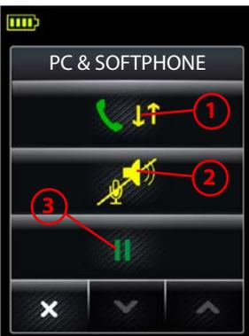
1. **Hold and switch:** touch here — or **press** the headset multifunction button — to put your current call on hold (at the back of the queue) and activate the first held call in the queue
