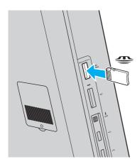
Before using "Memory Stick Micro" ("M2"), be sure to insert it into an "M2" Duo adaptor. If you insert the media directly into the "Memory Stick Duo" slot without the adaptor, you may not be able to remove it from the slot.
