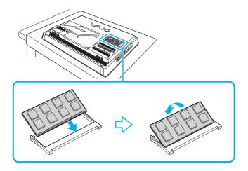
Do not touch any components on the motherboard other than the memory module.
