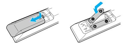
If your remote control does not operate properly, you may need to replace the batteries. When your remote control is not being used for extended periods of time, remove the batteries to avoid possible damage from battery leakage.
