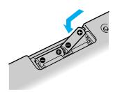
If your wireless keyboard does not operate properly, the batteries may need to be replaced. When your wireless keyboard is not being used for extended periods of time, remove the batteries to avoid possible damage from battery leakage.
