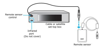
The remote sensor unit must be visible in a line-of-sight with your remote control in order to function properly.
