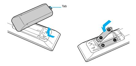
If your remote control does not operate properly, you may need to replace the batteries. When your remote control is not being used for extended periods of time, remove the batteries to avoid possible damage from battery leakage.
