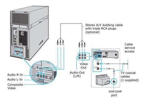
You can connect your computer to a set-top box using an S-video cable (optional) and an audio cable (optional) instead of a stereo A/V dubbing cable (optional). See "Connecting Other Devices."
