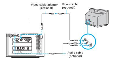
The video cable adapter is not necessary, if you use an S-video cable to connect your TV to the computer's TV out (S-video/video) jack.
