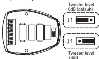
**Figure 8C.** Locating wiring connections on the GT0507C woofer. Other woofers are wired similarly.
