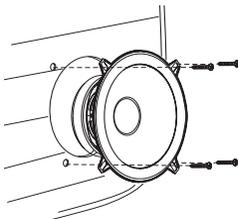
**Figure 2.** Mounting the woofer with the grille. (No grille is supplied with the GT08607C. It is designed to be installed under the factory grille.)
