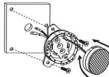
**Figure 7B.** Flush-mounted to surface behind grille panel.
