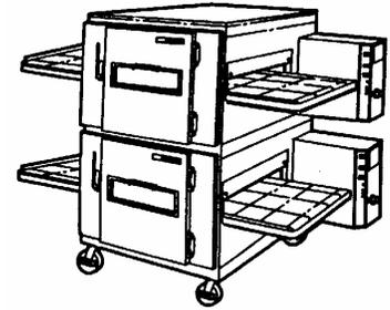
1. The stand is a 40" (1016 mm) x 49" (1245 mm) rectangle. Set it in place with a 40" side facing out. This will be the front of the oven. Using a carpenter's level, level all four (4) sides of the stand. To raise or lower the stand use the leg adjusters. Ovens on casters require a level floor. NOTE: The oven top is packed with oven stand. Remove top from stand before assembly.
