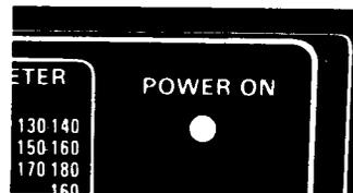
Any time the Selector for the single/upper or lower oven is turned to an oven function selection other than "OFF", the Power On Light will glow to tell you that the oven is turned "ON". The Oven Light, however, will come on and off in conjunction with the cycling of the heating elements.
