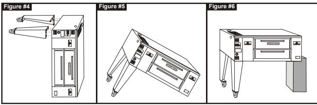
Mount other two legs and tighten bolts. Lift the oven and remove the supports.
