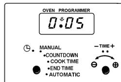
When you are using the minute minder you can make the clock show the time of day by turning the selector knob to 'manual'.
