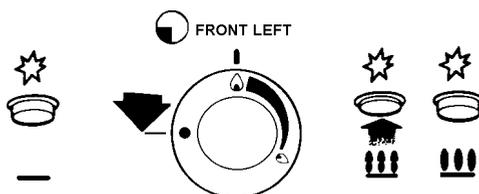
**Warning:** If the ignition button is not pressed immediately a build up of gas may cause the flame to spread.
