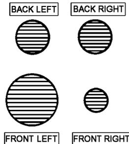
The largest pan which you should use on any burner is 230mm (9").
