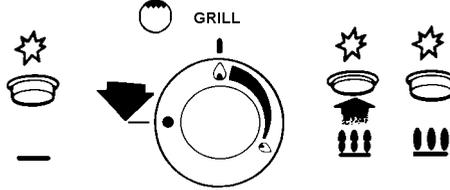
**Warning:** If the ignition button is not pressed immediately a build up of gas may cause the flame to spread from the grill cavity.
