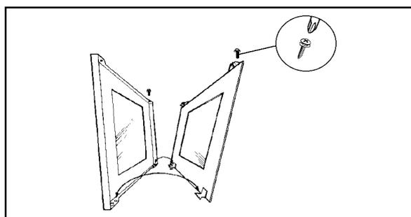
3. Hold the door panel securely in place with one hand before removing the screws completely with the other hand.
