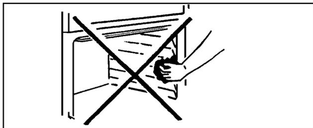
The vitreous enamel base in the grill compartment and the fan oven base can be cleaned using normal oven cleaners or aerosol oven cleaners with care. Ensure that the manufacturers instructions are followed and that all parts are well rinsed afterwards.
