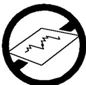
**Do not** use the cooker if the ceramic glass is damaged. If a fault or crack becomes visible during cooking, disconnect the cooker immediately from the electricity supply and contact your local Service Force Centre. **Do not** place silver foil or plastic containers on ceramic glass.
