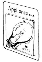
3. Replace the bulb with a 40-watt **appliance** bulb available from most grocery, variety and hardware stores. Turn electrical power back on at the main power supply.
