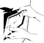
fip the window and frame out from the top slightly
