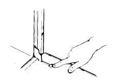
Open the door. Swing broil stop clips over hinge slots.
