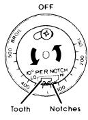
**3.** To lower the temperature, move black ring so tooth is closer to LO. Each notch equals about 10 F (5 C).
