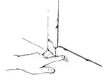
When the hinges snap into place, open the door and move the broil stop clips. Close the door.
