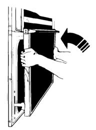
Hold the door on both sides. Tip in on the top and lift slightly.
