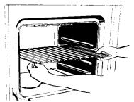
1. Put rack in broiling position (see below). put broiler pan and tood on the rack
