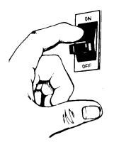
1. Turn off the electric power at the main power supply.
