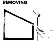
With the door closed, remove the screws from the top of the outer window trame
