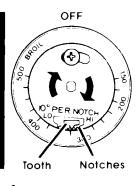
4. To raise the temperature, move black ring so tooth is closer to HI. Each notch equals about 10 F (5 C).
