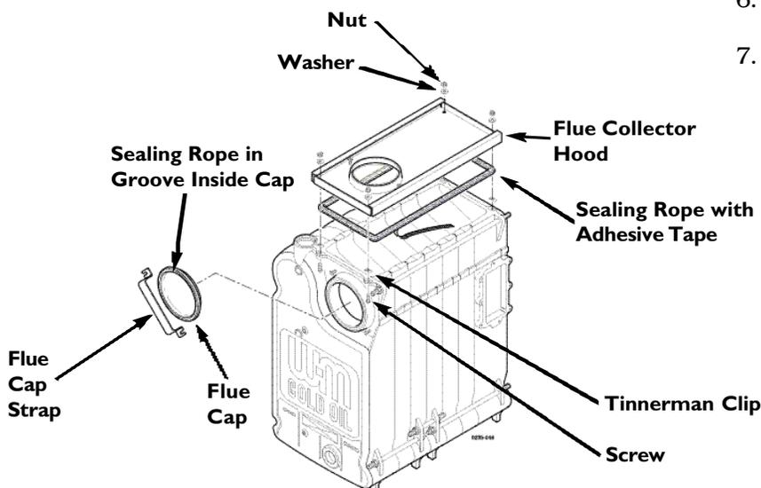
Change from Back Flue Outlet to Top Flue Outlet (Optional)
