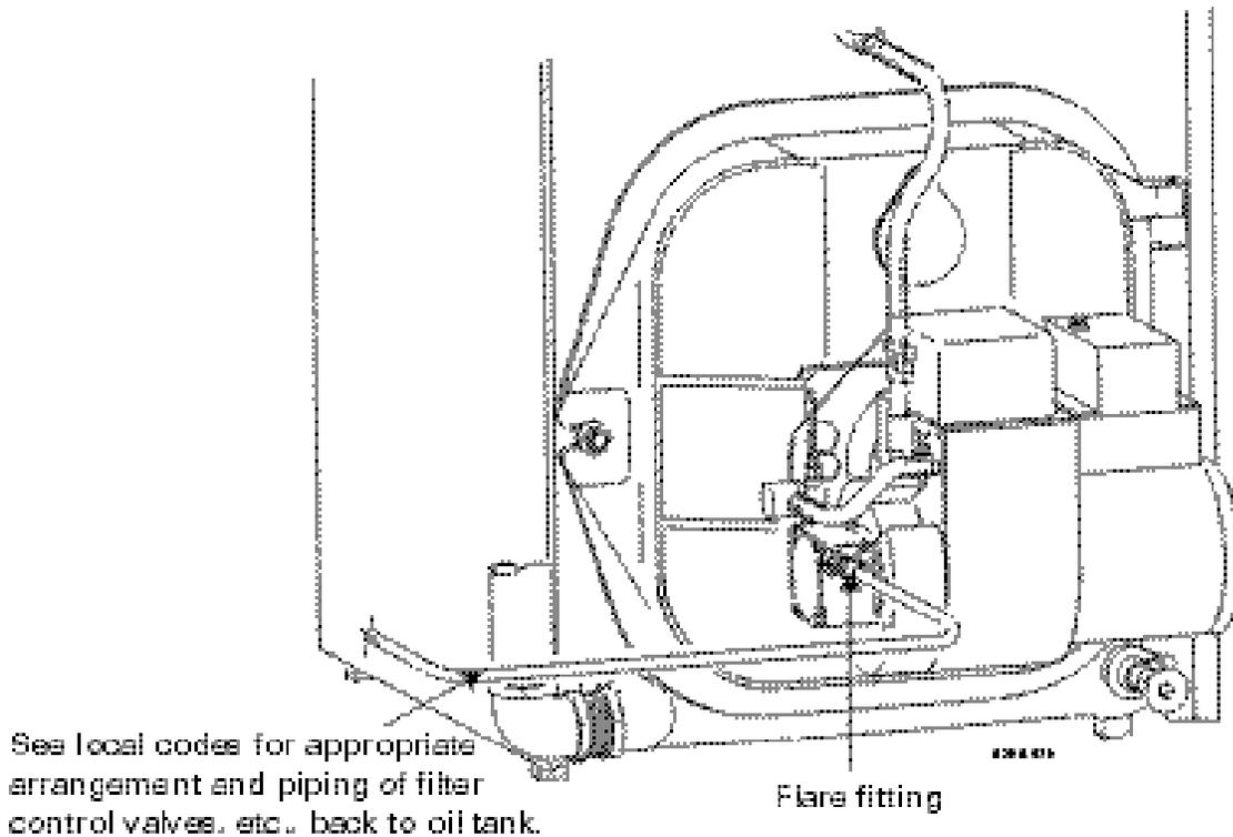
Recommended Oil Piping Connection to Burner
