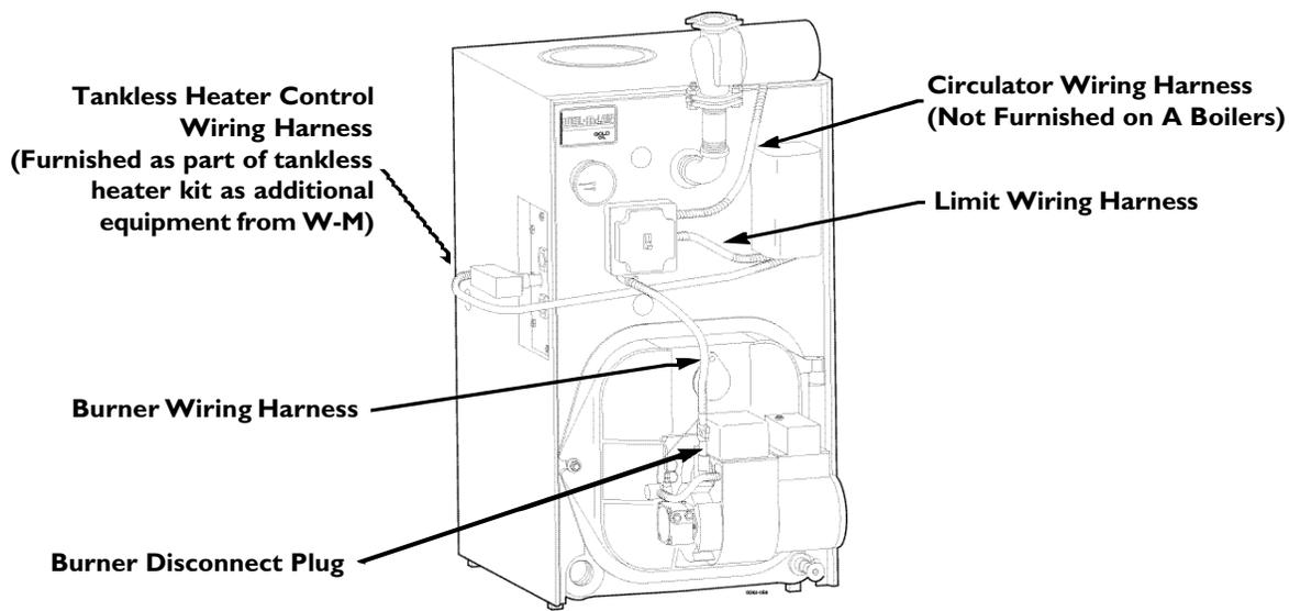
Boiler Wiring for Forced Hot Water
