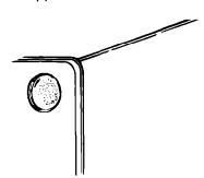
Replace the bulb cover by screwing it in clockwise. Reconnect appliance at the main power supply.
