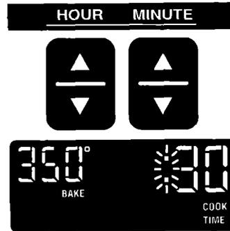
5. Push the Start/Enter pad. “Lo”, HEAT, BAKE, TIMED, and the set cook time will show on the display to indicate that the oven is heating.
