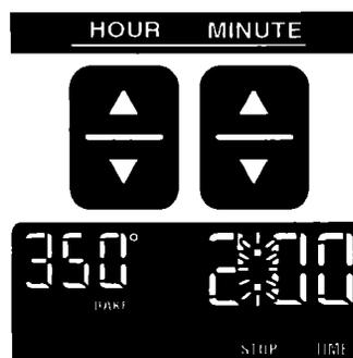
This example shows a desired stop time of 2 o'clock. This provides a 2-hour cook time (the difference between the time of day and the stop time).
