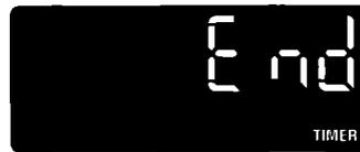
**NOTE:** To disable the reminder tones, push and hold the Timer Set pad for 4 seconds. To reactivate the tones, follow the same procedure.
