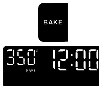
3. Push the Stop Time pad. The time of day with the colon flashing and STOP TIME will show on the display.
