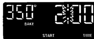
5. **Push** the Stop Time pad. The time of day with the colon flashing will show on the display and STOP TIME will light up.
