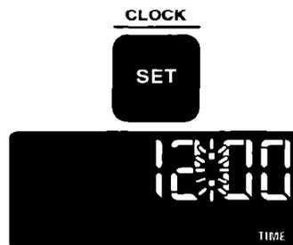
2. Use the Hour and Minute pads to set the time of day. Push the "up" (▲) or "down" (▼) pad(s) until the correct time shows on the display.
