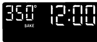
3. **Push** the Delay Start Time pad. The time of day with the colon flashing will show on the display and START TIME will light up.
