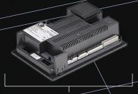
The Ultra Control Module, a microprocessor electronic control, responds to signals from the room thermostat, supply water temperature sensor, return water temperature sensor, flue temperature sensor, domestic hot water aquastat, summer/winter switch and outdoor temperature sensor. The module automatically adjusts blower speed and gas flow rate to modulate boiler firing rate to closely match beiler output for space heating or DHW heating demand.
