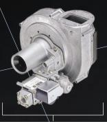
The blower, gas valve and venturi all work in concert to provide the proper fuel and air mixture for precise combustion. The blower pulls in air and gas through the venturi. The air and gas mix inside the blower and are pushed into the burner for combustion. The gas valve senses suction from the blower, allowing gas to flow only if combustion air is flowing and proper combustion is achieved.
