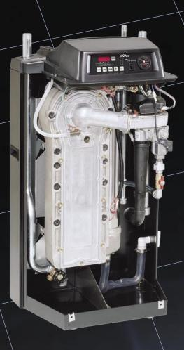
High grade stainless steet burner with woven steel fiber mesh. Burner uses pre-mixed air and gas providing for a 20% to 100% modulating firing rate. The Ultra burner features long life, quiet operation, high efficiency and cleaner combustion for low NOx applications.
