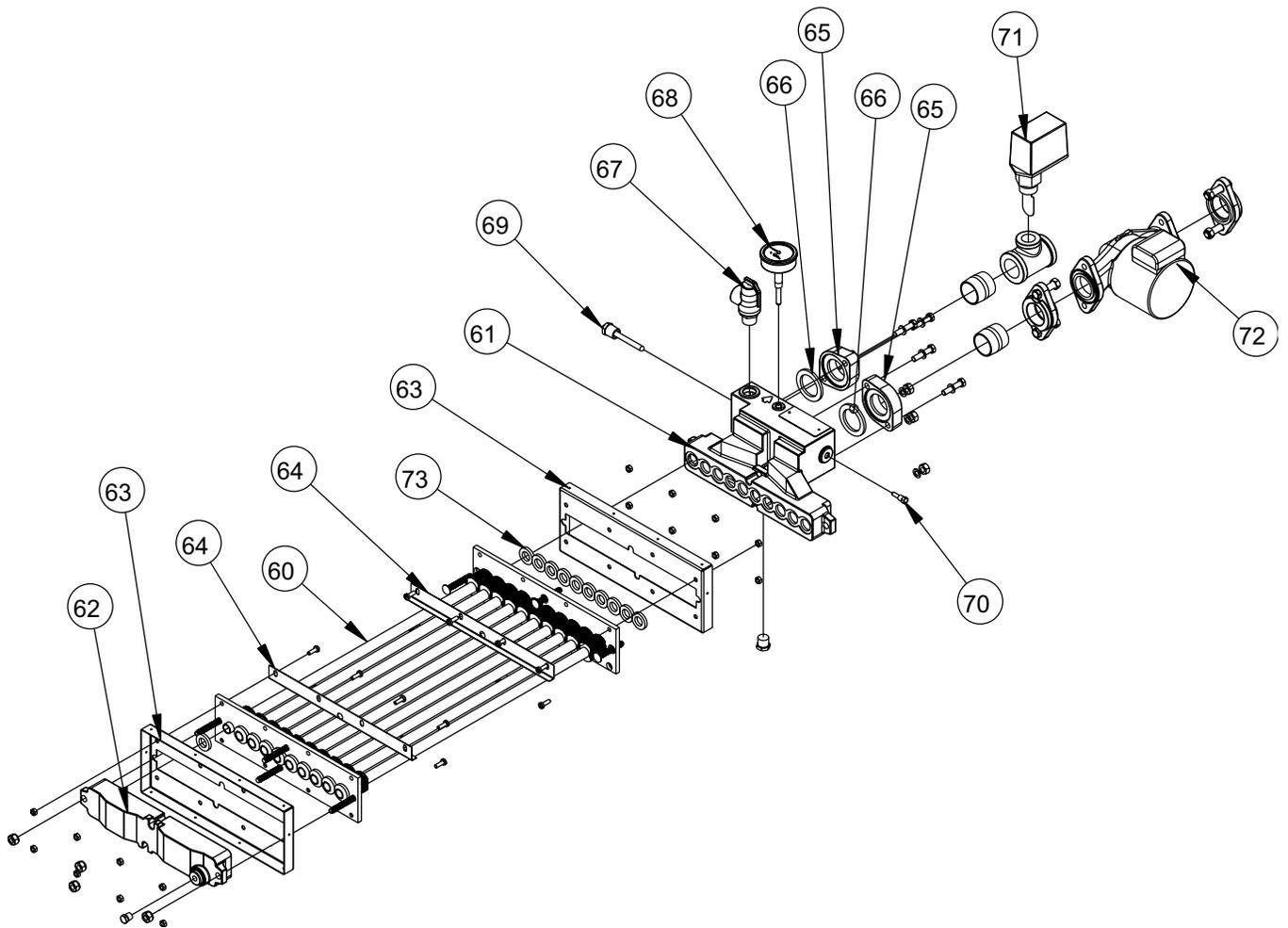
Figure 22. Heat Exchanger Components.
