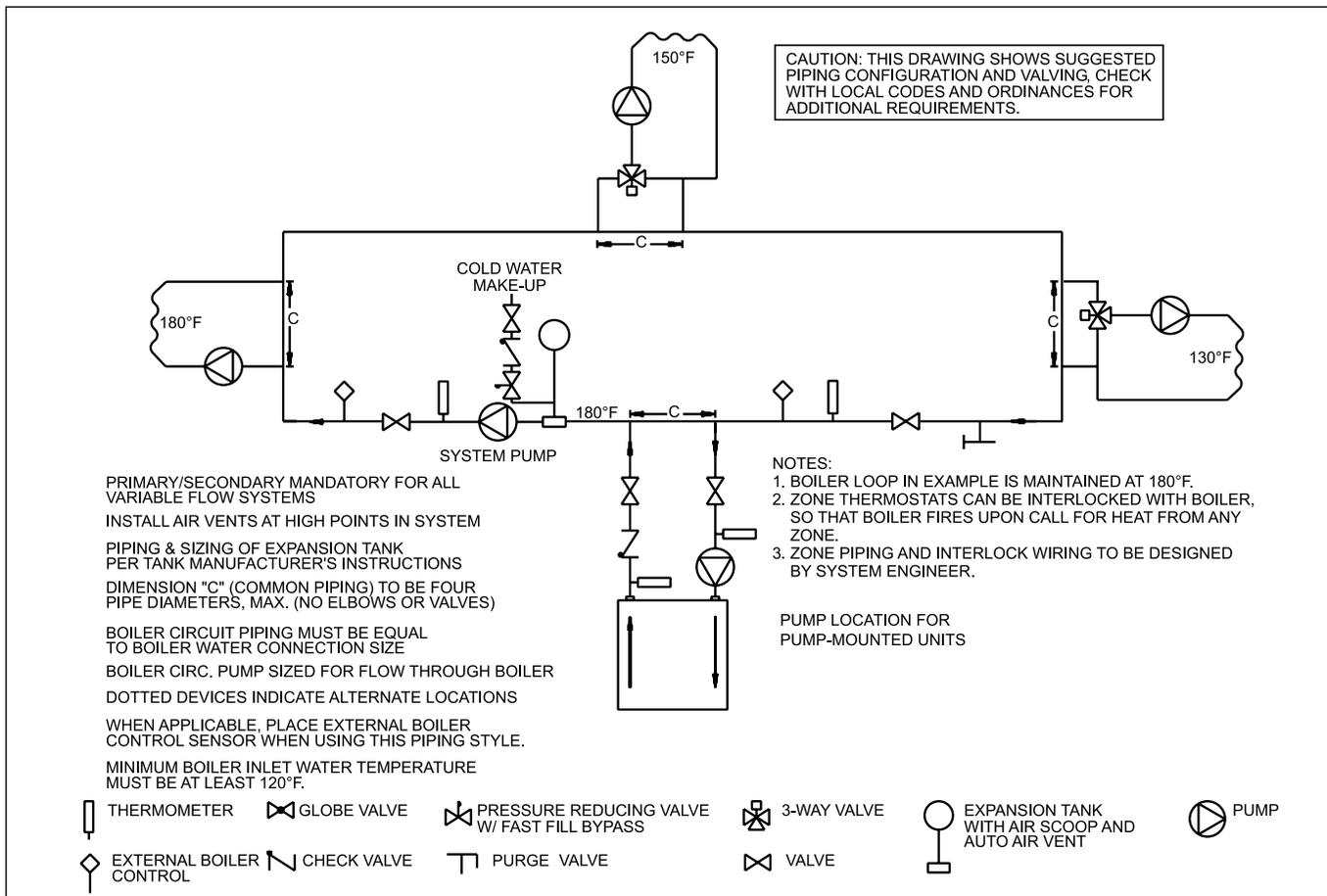
Figure 6. Hydronic Piping — One Boiler, Multi-Temperature System.
