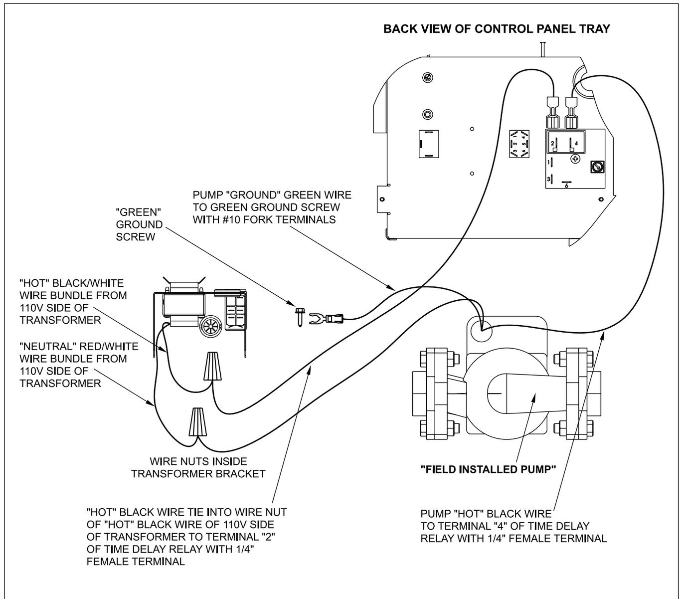
Figure 14. Field Wiring.
