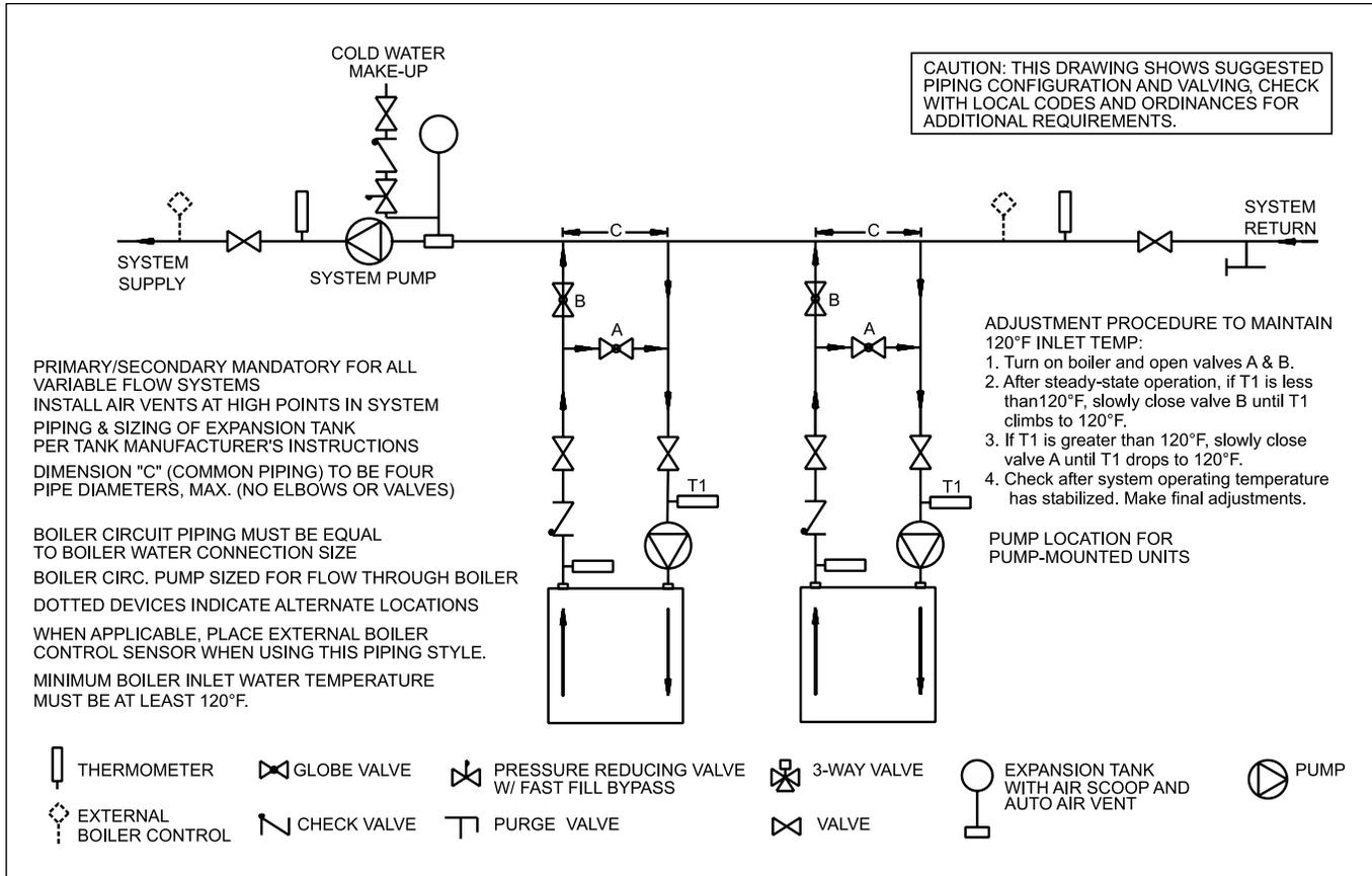
Figure 5. Hydronic Piping — Multiple Boilers, Low Temperature System.
