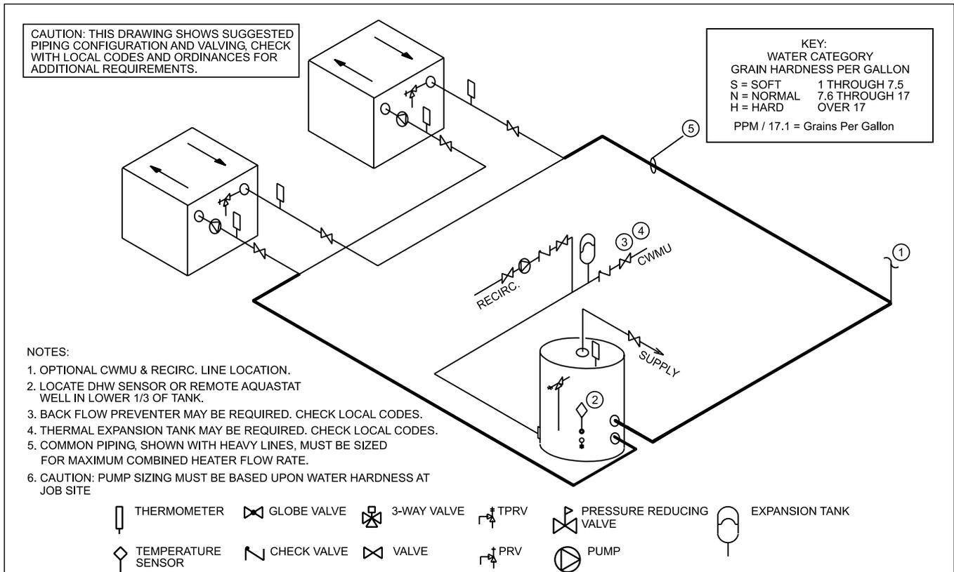
**Figure 10. Water Heater Piping — Multiple Heaters, One Tank.**
