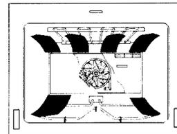
With the selector set to convection cook and the temperature control on 150 F, warm air is circulated by a motorized fan in the rear of the oven. Over a period of time, the water is removed from the food by evaporation. Removal of water inhibits growth of microorganisms and retards the activity of enzymes. It is important to remember that dehydration does not improve the quality, so only fresh, top-quality foods should be used.
