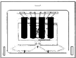
In Maxi-Broil heat is radiated from both broil elements, located in the top of the oven cavity, at full power. Broiling speed is determined by the distance between the foods and the broil elements. For "fast" broiling, food may be as close as 2 inches to the broil element or on the top rack. "Fast" broiling is best for meats where "rare to medium" doneness is desired. The Mini-Broil setting is designed for "slow" broiling. Only the center broil element operates for partial power.
