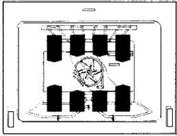
Full power heat is radiated from the bake element in the bottom of the oven cavity, and supplemental heat is radiated from the broil element. This function is recommended for single rack baking and roasting.
