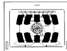
This oven features a pyrolytic self-cleaning cycle. During this cycle, the oven reaches elevated temperatures in order to burn off soils and deposits. An integral smoke eliminator reduces odors associated with the soil burn-off. A powder ash residue is left in the bottom of the oven after completion of the self-clean cycle. When the oven has cooled, remove any ash from oven surfaces with a damp sponge or cloth.
