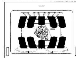
With the selector set to convection cook and the temperature control off, air is circulated by a motorized fan in the rear of the oven. The fan accelerates natural defrosting of the food without heat. To avoid sickness and food waste, do not allow defrosted food to remain in the oven for more than two hours.
