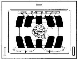
Exactly the same as regular baking with the additional benefit of air circulation. The heated air is circulated by the motorized fan in the rear of the oven. It provides more even heat distribution throughout the oven cavity for all uses. Multiple rack use is possible for the largest baking jobs. When roasting, cool air is quickly replaced-searing meats on the outside and retaining more juices and natural flavor on the inside with less shrinkage.
