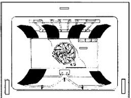
The rear element only operates at full power. There is no direct heat from the bottom or top elements. Air in the oven cavity is circulated by the fan for even heating. Use this setting for foods which require gentle cooking such as pastries, souffles, yeast breads, quick breads and cakes. Use this function for single rack baking, multiple rack baking, roasting, and preparation of complete meals.
