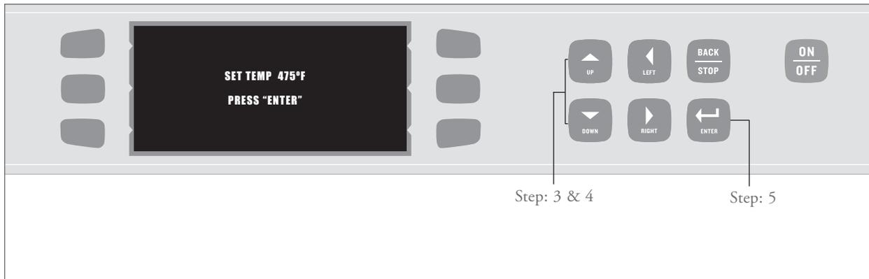
FIGURE 14: Adjusting the Cook Chamber Temperature
