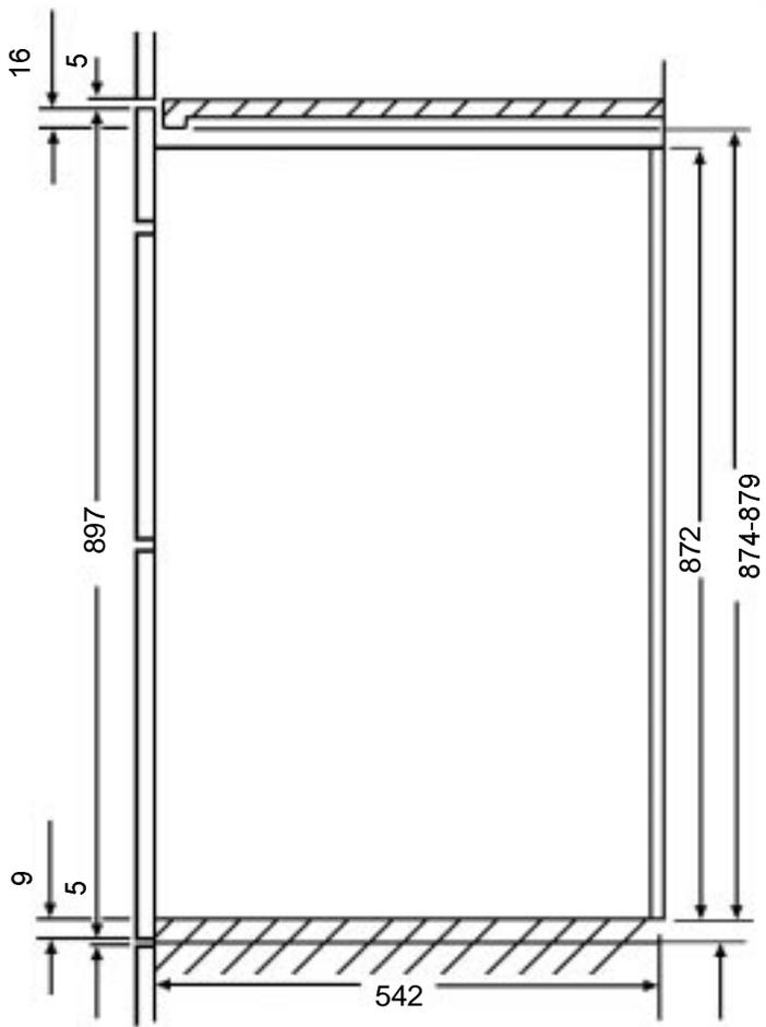
**Cross section through cabinet showing oven positioned**
