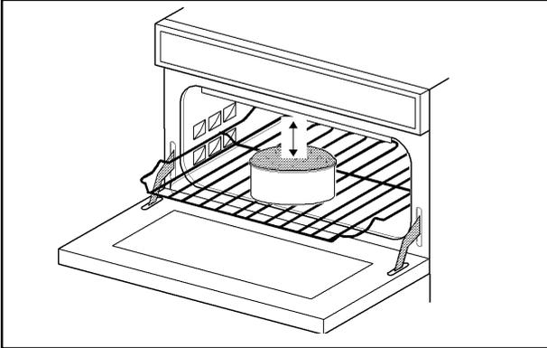
Dishes, tins and trays should not be placed directly on oven floor as it becomes very hot and damage will occur.
