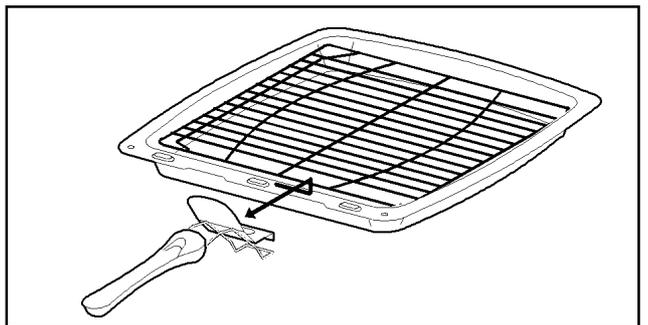
Place the grill pan on the shelf so that the pan is positioned centrally beneath the grill.
