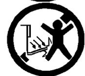
Stand clear when opening the drop down oven door. **Do not** allow it to fall open - support it using the door handle, until it is fully open.
