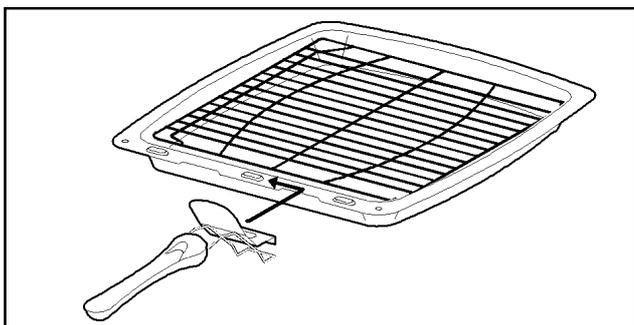
**Ensure the handle is correctly located. It is not necessary to remove the grill pan handle during grilling.**
