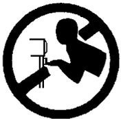
**Do not** try to *lift* or move the appliance by pulling the door handles. Refer to installation instructions.
