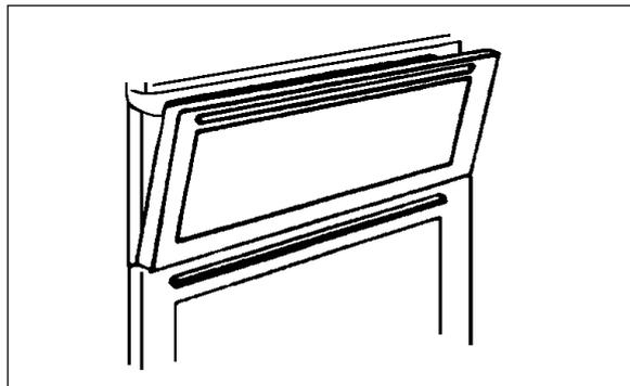
2. Holding the oven glass with both hands, gently place the locators into the holes of the brackets at the bottom of the oven door.
