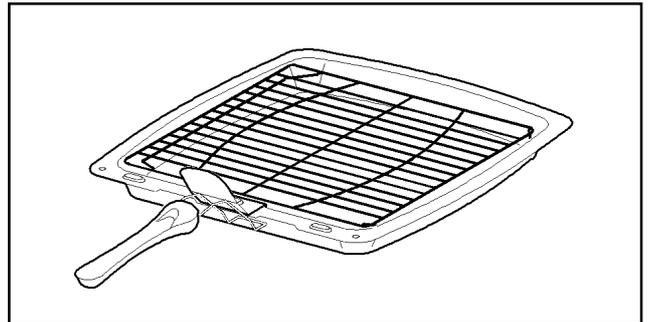
To remove the handle, slide the handle to the right and lift the handle away from the cut out on the grill pan.
