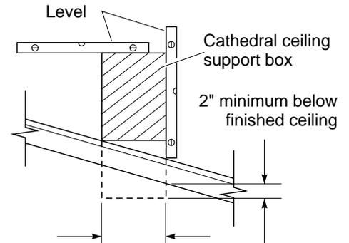
Cut hole 1/8" larger than support box when projected onto roofline
