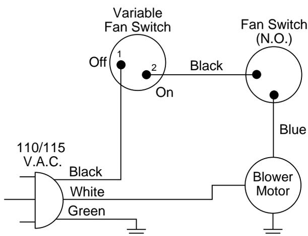
Figure 63 - Blower Wiring Diagram for Thermostat-Controlled Models
