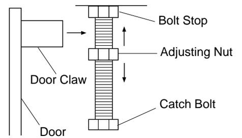
**Figure 13 - Catch Bolt and Door Claw Orientation**
