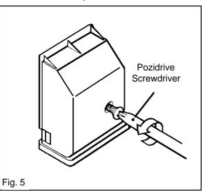
Prise cover loose using screwdriver in position
