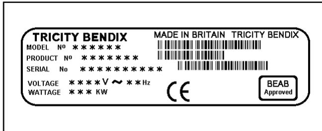
The cooker must be protected by a suitably rated fuse or circuit breaker. The rating of the cooker is given on the rating plate.
