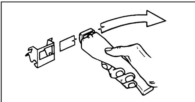
To correctly locate the grill pan on the shelf, ensure that the cut out on the underside of the handle bracket locates over the front bar of the shelf.
