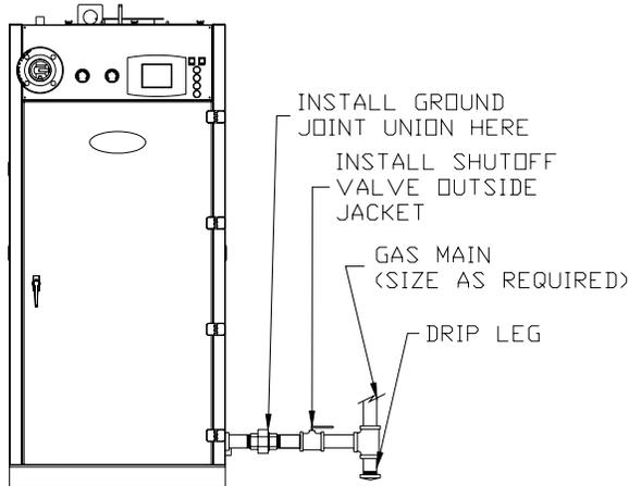
Figure 2 Main Gas Inlet Connection
