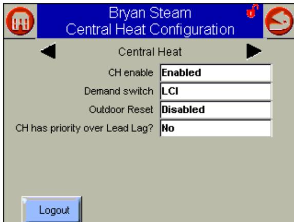
Figure 36 Central Heat Configuration (Central Heat Page)
