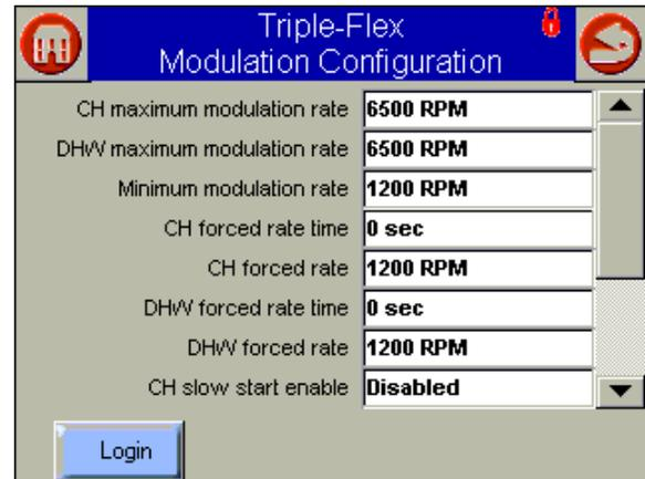
Figure 27 Modulation Configuration
