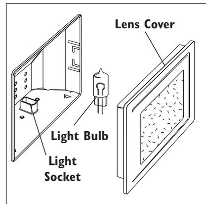
3. Support the glass lens cover with two fingers along the bottom edge to prevent the cover from falling to the bottom of the oven.
