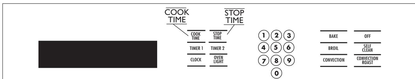
The oven has a provision for locking the control panel in the **OFF** position. This mode prevents accidentally turning on the oven while cleaning the control panel or from a child playing with the pads. Oven modes which are locked **OFF** are **BAKE, CONVECTION, CONVECTION ROAST, BROIL** and **CLEAN** for both ovens, if a double oven is being used. The functions which can always be used regardless of a lockout are: **TIMER 1** or **2, CLOCK,** and the oven **LIGHT**.
