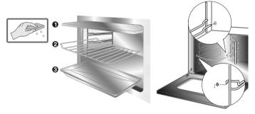
Clean the oven shelves with hot water and non-abrasive detergents, rinse and dry. For easier cleaning, the door can be removed (see point "14.2 Removing the door")
