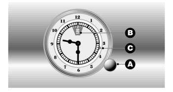
The cleaning cycle can be programmed so this begins at a preset time. Turn the knob **A** anticlockwise to set duration of pyrolysis in window **B**. **PULL** and turn the knob **A** anticlockwise so the arrow **C** coincides with the desired start time.
