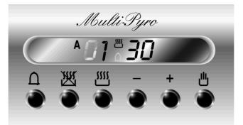
The cleaning cycle can be programmed so it starts at a specific time. Press key  $\[mu]$  and change the setting by means of setting variation keys - or +.
