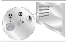
Remove the bulb protector A by turning it anticlockwise and replace bulb B with a similar one (25 W). Re-fit the bulb protector A.
