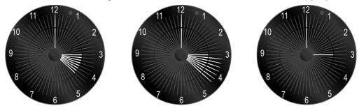
The start of the pyrolysis cycle can be programmed within the next 12 hours. After setting the pyrolysis duration, press the  $\underbrace{III}_{}$  key and set the pyrolysys start time by pressing the -/+ keys. The internal segments will remain on and the external ones will flash until the current time is the same as the cycle start time. The process will now start and the segments will start to flash as already described.
