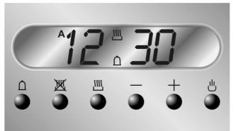
The cleaning cycle can be programmed to start at a preset time. Press the  $\underline{W}$  key and adjust the values using the value variation keys – or +.
