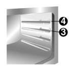
Ensures quick browning of food. The plate is best inserted at top level. For short or small-quantity cooking, the rack should be (A) inserted at the third level from the bottom. For longer cooking and wide-surface grilling, fit the rack at bottom level. This will also depend on size of food.
