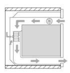
The oven features cooling fans which switch on together with the oven.
