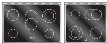
The 4/5 signal lamps located between the cooking zones come on when the temperature of one or more of the heating zones exceeds 60°C. The lamps go off upon temperature dropping to below approximately 60°C.
