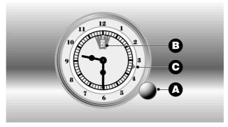
The cleaning cycle can be programmed to start at a preset time. Turn the knob **A** anticlockwise to set the Pyrolysis duration in the window **B**. **PULL** the knob **A** and turn it anticlockwise until the arrow **C** is in line with the cooking start time required.
