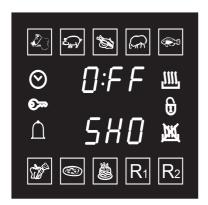
**Showroom mode:** (only for showrooms) by activating this mode, the oven deactivates all the heating elements, while keeping the control panel active. To use the oven normally, set this mode to OFF. During cooking, the word SHO will be displayed (once per minute) to indicate that the showroom mode has been activated.
