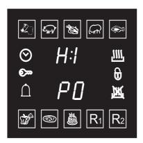
Power limiter mode: by selecting LO while cooking with the main oven a limited amount of power will be used, according to the model. To reset the product's normal consumption, select HI.
