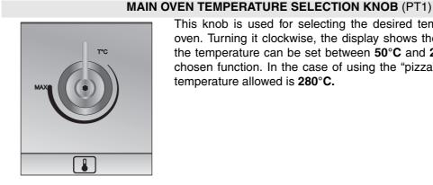
This knob is used for selecting the desired temperature for the main oven. Turning it clockwise, the display shows the temperature just set, the temperature can be set between 50°C and 260°C according to the chosen function. In the case of using the "pizza" recipe, the maximum temperature allowed is 280°C.
