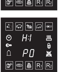
Power limiter mode: by selecting LO while cooking with the main oven a limited amount of power will be used, according to the model. To reset the product's normal consumption, select HI.
