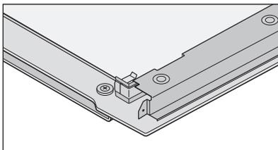
3. Attach glass #1, the door bracket and the supports to the door.
