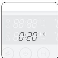
**3** Press the **Cook Time Button**. The oven operates with the selected cook time unless the **Cook Time Button** is pressed within 5 seconds.
