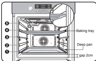
The baking tray, deep pan and wire grill should be inserted correctly into the side runners. When taking out the cooked foods from the oven, be careful of hot utensils and surfaces.
