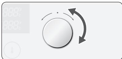
**3** Turn the **Time / Temp Control Knob** to select the desired oven function. If 3 seconds have elapsed and there are no further adjustments, the oven will begin automatically in the selected mode and function.
