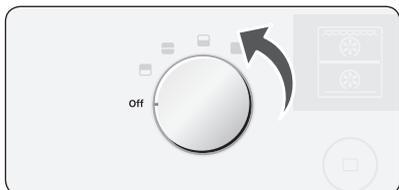
To switch the oven off, turn the **Divider Select Knob** to the "Off" position.
