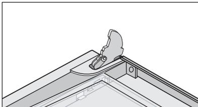
2. Attach the two spring brackets at the top of glass #2 and place glass #2 into position.
