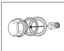
4. Fit the metal and the sheet ring to the glass cap.
