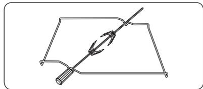
**6 Rotisserie spit** (BT62CDBFST) comprises a spit, 2 prongs, a removable handle and a cradle, which fits into the 3rd shelf from the bottom. To use the rotisserie, fit the spit into the hole in the rear wall of the oven's interior. Place the deep pan on level 1 when using the spit.
