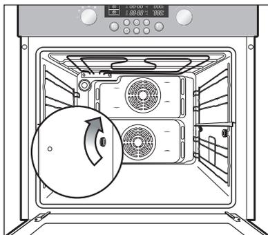
2. Insert and push the back U-form of the side runner towards the screw.
