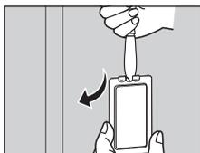
1. To remove the glass cover, hold the lower end with one hand, insert a flat sharp implement such as a table knife between the glass and the frame and pop out the cover.
