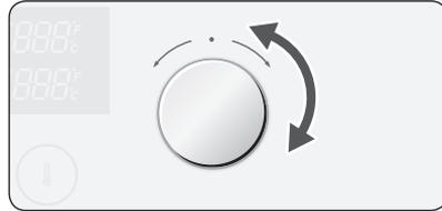
**2** Turn the **Time / Temp Control Knob** to adjust the temperature in increments of 5 °C.
