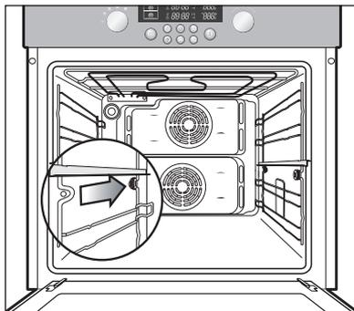
3. Insert the screw at the front, and fasten both screws.
