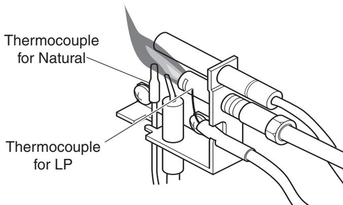
**Figure 17 - Correct Appearance of Pilot Flame**
