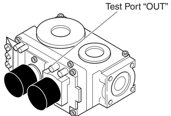
**Figure 11 - Pressure Test Point Location
