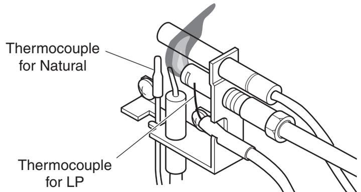
**Figure 18 - Incorrect Appearance of Pilot Flame**
