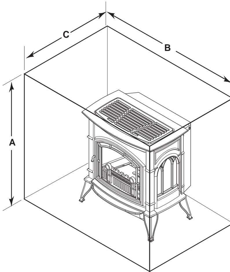
**Figure 6 - Placing Stove in Alcove**
