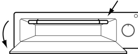
2. Cut the nylon straps. Remove nylon straps and Door Handle from unit.
