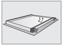
■ Refit the glass fibre seal.
