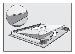
■ Replace the first of the middle panes. The more angled corner must be at the bottom left. When refitting the upper pane, the more angled corner must be inserted at the top left.
