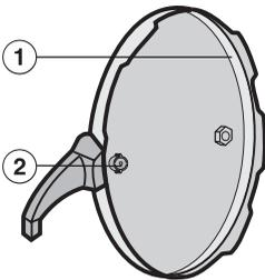
Depending upon frequency of use, the door seal ① and the safety valve ② should be replaced every 1-2 years. Replace both parts at the same time.
