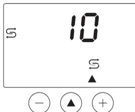
The number indicates that the appliance can be used a further 10 times before it locks out. If the appliance is not descaled immediately, a
