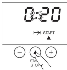
"Start" will appear in the time display, the  $\Rightarrow$  symbol will stop flashing, and the colon will begin to flash.
