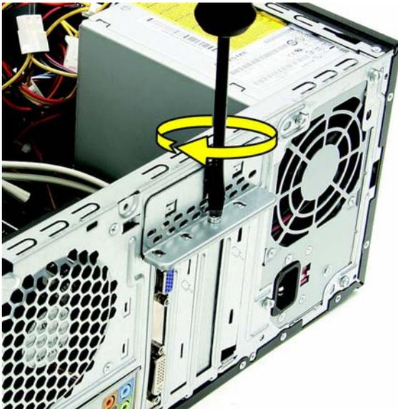
18. Connect external cables to the installed card, if needed. Connect internal cables to the system board, if needed.
