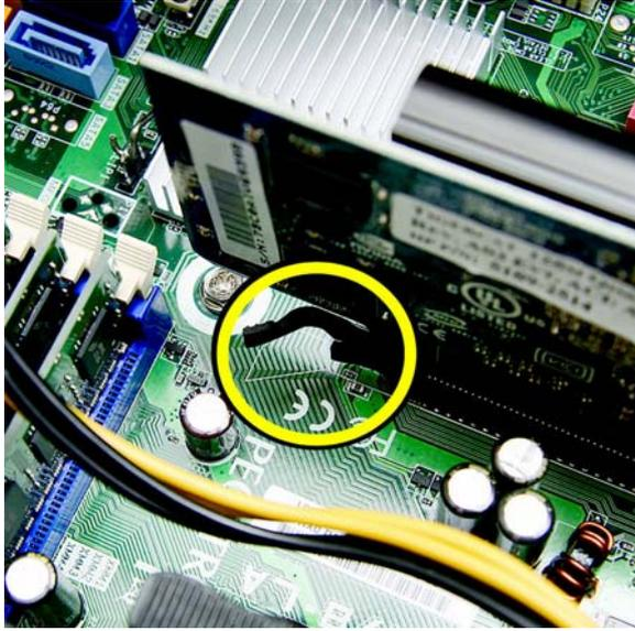
15. Press straight down until the card is fully seated in the card slot.
