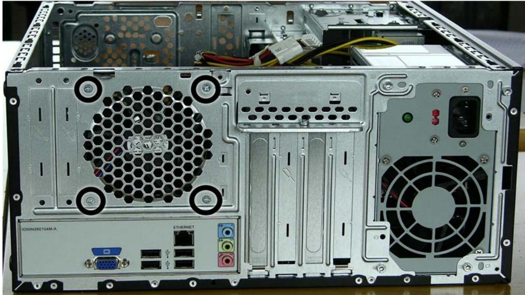
To install the fan, reverse the removal procedures.
