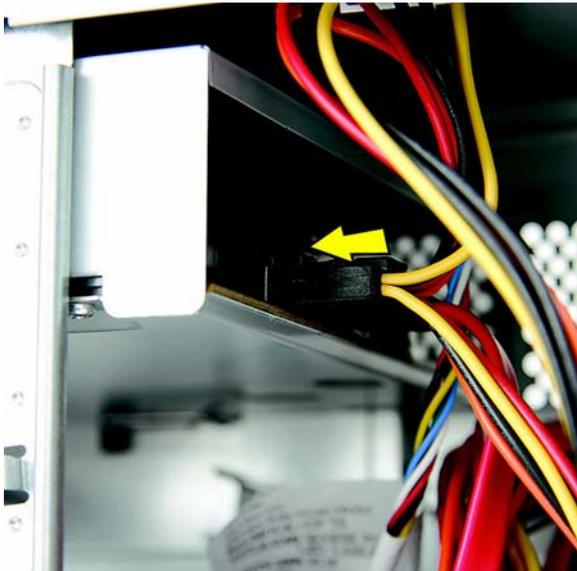
7. Align the disc drive screw holes with the drive bay holes (marked “2”).
