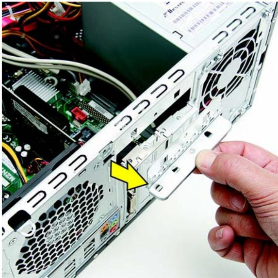
6. If you are removing a graphics card, press on the latch to release it.
