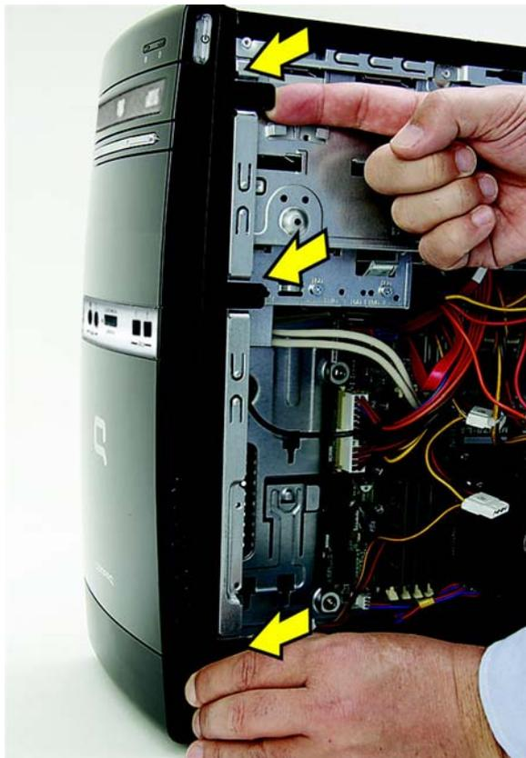
4. Swing the front bezel out to remove from the computer.
