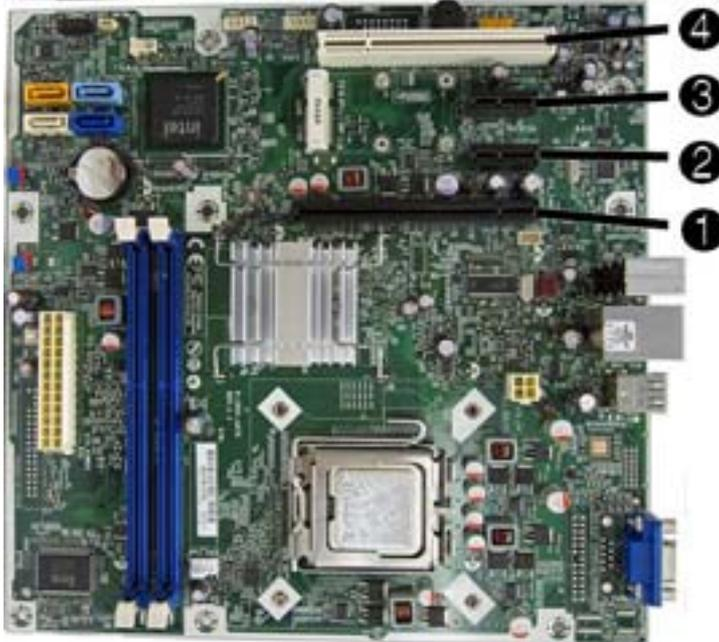
**Figure 2-11** Expansion Slot Locations — 505B/515B
