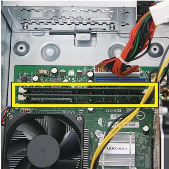
4. Open both latches of the memory module socket (1), and insert the memory module into the socket (2).
