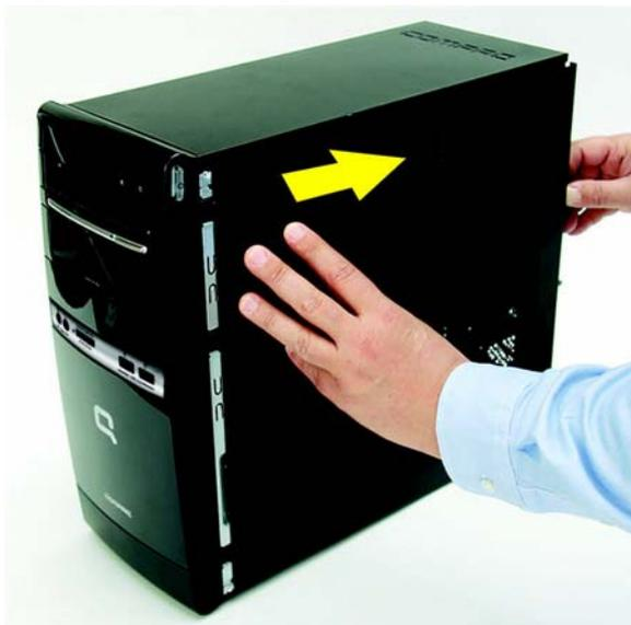
4. Remove the side panel by lifting it away from the computer.
