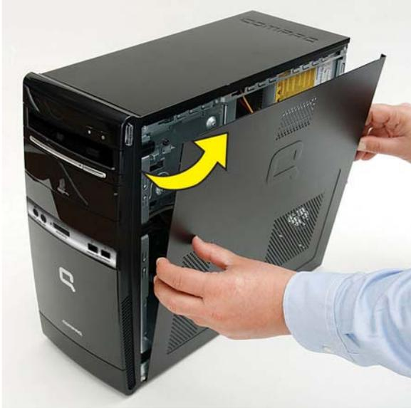
To replace the access panel, reverse the removal steps.
