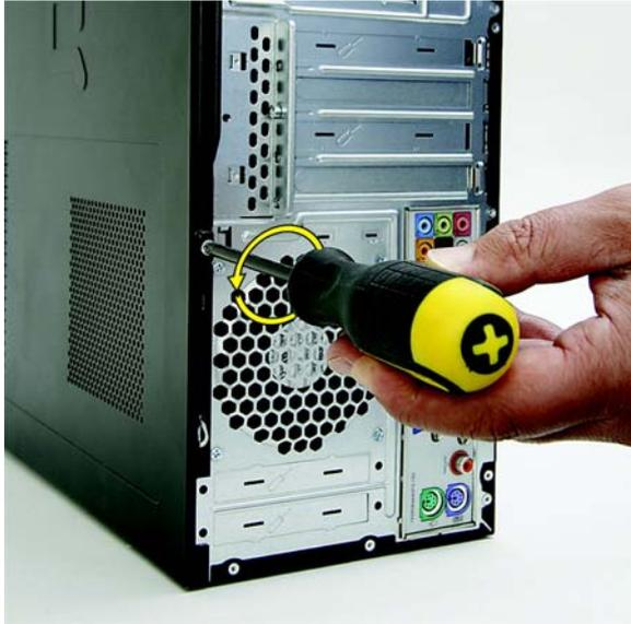
3. Grasp the handle on the side cover and pull towards the back of the computer. Slide the cover about 2.4 cm (1 inch) to remove it.
