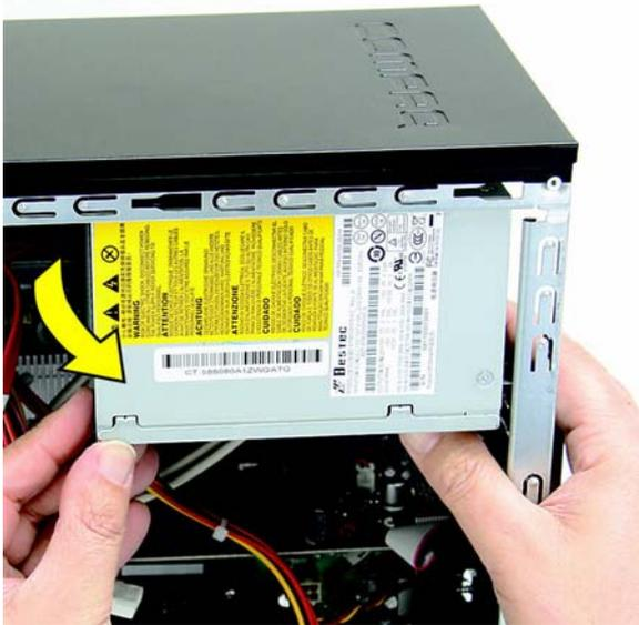
To install the power supply, reverse the removal procedure. Note that there is a latch, a guide, and a ledge on the computer that help secure the power supply.
