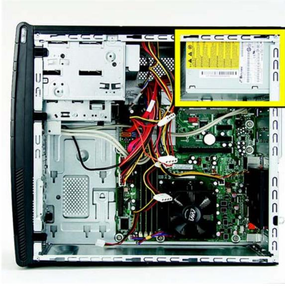
**NOTE:** Noting the location, type and orientation of the power connectors is extremely important. Failure to correctly restore all power connectors appropriately will prevent the computer or components from working successfully.
